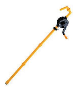
With Teflon seal, Ryton vane, PP spout,, PP suction tube. The outlet can be freely adjusted from 0° to 360° Applicable Liquids: acid, alkali, gasoline, diesel, machine oil, water, alcohol, thinner, and other chemical liquids. PATENTED IN TAIWAN, CHINA, FRANCE.
