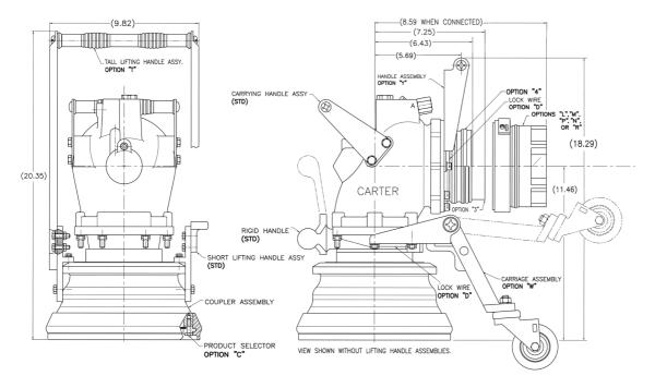
Various options are available on Model 64910 coupler. The complete model number is comprised of four parts, as explained in the tables below.
