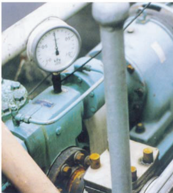
PFM Valve fitted to V40 Pump
