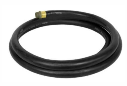
1 x 12' fuel transfer hose with internal spring guard, stainless steel ground wire and fuel-resistant neoprene exterior. Designed for gasoline, diesel, B20, E15 and kerosene. Suitable for all electric pumps.
