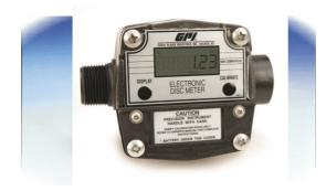
Lightweight, corrosion resistant high-tech injection molded plastic housing. Reliable nutating dsc measuring chamber. Advanced encapsulated environmentally protected electronic circuitry for high accuracy. Display rotatable in 90deg increments.
