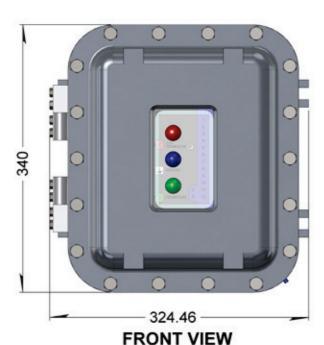
MOUNT WITH 4 OFF M12 OR 1/2" FASTENERS MOUNTING DIMENSIONS X
