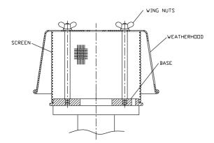
**Sizes Available.** 2" (DN 50) through 12" (DN 300) aluminum units flanged to mate with 125# ANSI and DIN PN 16 flat face flanges. All other materials mate with 150# ANSI and DIN PN 16 raised face flanges. 16" (DN 400) through 24" (DN600) units flanged to mate with applicable ANSI or API flat face flange connections.
