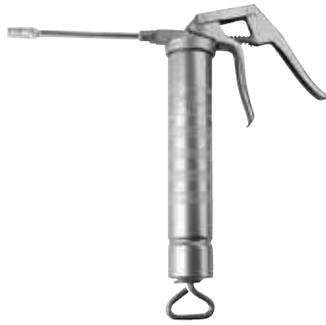
Pistol grip grease pump for hard to reach lubrication points. Three way loading: 400 g (14 oz) cartridges, bulk grease suction or filler pump. Heavy duty cast iron head with precision fit piston. Maximum working pressure: above 250 bar (3,650 psi).
