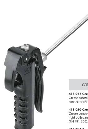
High pressure grease control guns with ergonomic body and trigger designed to reduce operator hand fatigue. Manufactured in aluminium with steel insert for high pressure. Maximum working pressure: 500 bar (7,150 psi). Inlet thread: 1/4" BSP (F).
