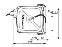
Compact enclosed reels for air, manufactured in steel. All reels include pivoting wall bracket for an easy and convenient installation. Reels include polyurethane and PVC hose with a maximum working pressure of 15 bar (285 psi)
