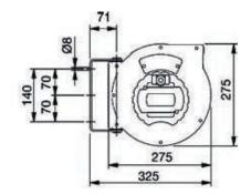
Compact reels with high resistance thermoplastic enclosure. Compact design, with wide outlet for a comfortable friction free cable extension. All reels include pivoting bracket, cable specified for each model, and cable overload breaker.
