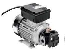
Internal gear electric pumps for lubricants. 230 V - 50 Hz (single phase) or 380 V - 50 Hz (three phase) motor depending on model, IP-55 protection and on/off switch. Cast iron pump body, sintered steel gears and by-pass valve. Motor with mounting feet, the pump can be mounted horizontally on a flat surface or vertically to a wall.
