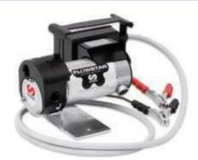
External gear pumps with 12 and 24 V DC motors wit IP55 protection, on/off switch, fuse and 2 m cable with crocodile clamps. Pump can work in interment duty cycles of 30 minutes and has built in by-pass valve.
