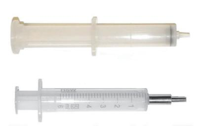
In order to perform the Water Detection test we offer a series of re-useable 5ml syringes. Low cost medical specification syringes should not be used for the test because they often have the incorrect tip size which will not fit the water detector capsule, and they may have an extremely short service life.
