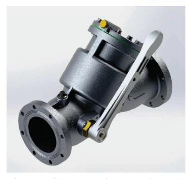
The main parts of the coupler are made in aluminium alloy. Standard seals in fluoroelastomer FPM-NT (Viton®) are easy to maintain. The surfaces subject to wear are hard coated.
